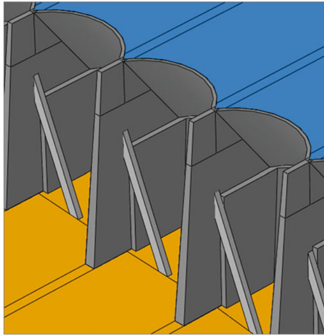
Fig. 25.10 Flying buttress concept applied to FEM (subset shown, buttresses applied to all arches)
